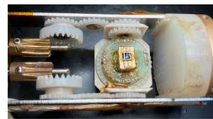
Fig. 1: A photograph of two-axis rotator for high-field magnets in IMR.
